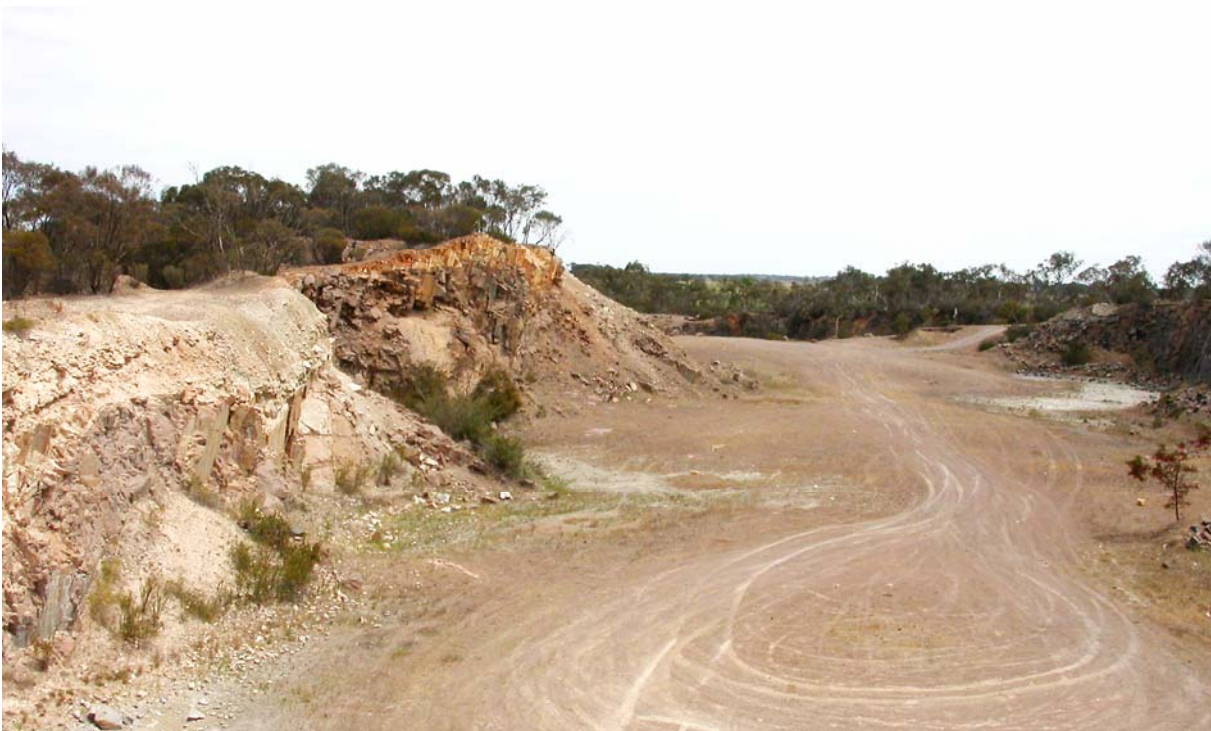
Plate 2. Mount Monster Northern Quarry, view west-southwest from top of eastern face. Weathered rhyolite of variable depth overlies fresher rhyolite in southern face.
